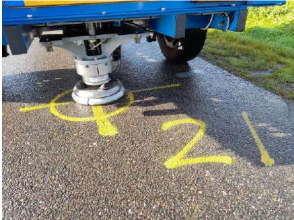
Figure 3 Positioning of loading plate in circle at test station 121 and 221 (2021)
